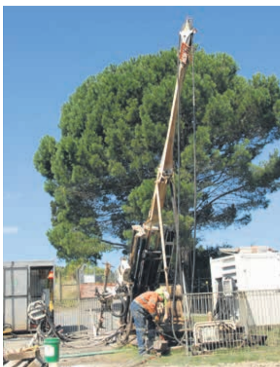
One of three exploration drill rigs currently working on the pit rim.
