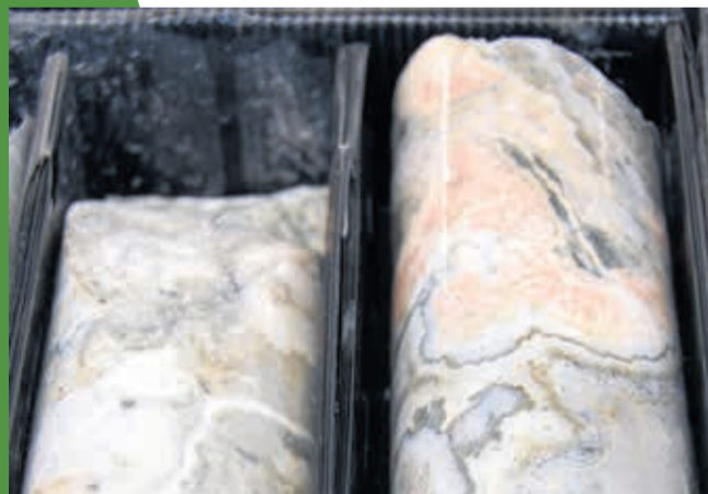
Drill core showing quartz veins with sulphides (the dark spots and bands) and inesite (pink) manganese zeolite for which Waihi is the 'type locality' in the world.
