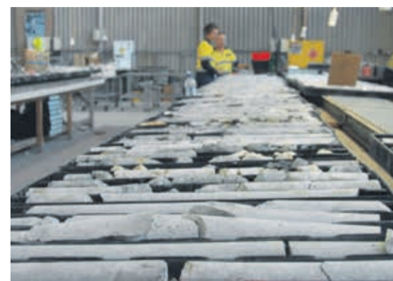
Core received from the drill rigs is logged and analysed at the core shed.
