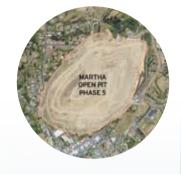
involves cutting back the Martha pit around its full circumference. The pit would generally be about 40 metres deeper, 160 metres longer and 80 metres wider than the existing Martha pit. Surface mining operations would be by conventional drill, blast, load, and haul methods.
