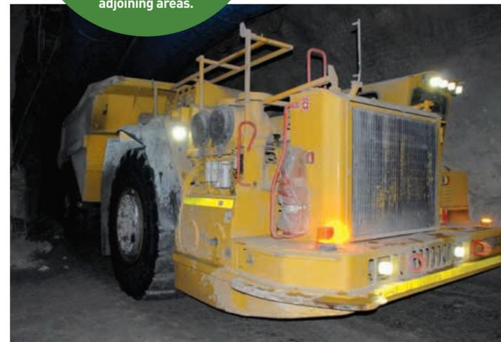
Low profile underground trucks will haul ore to the surface via the existing Favona portal and cart surplus material underground to be used as backfill.
