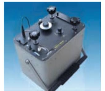
A portable gravimeter detects minute changes in gravity.
