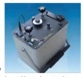
A portable gravitometer detects minute changes in gravity.
