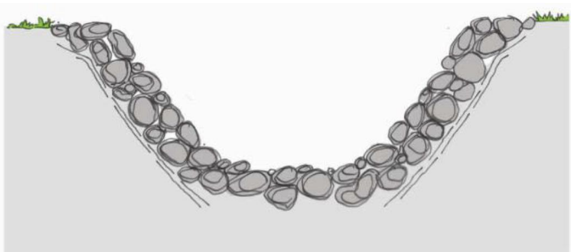
Rock-Lined Flow Channel for High Flow and/or Steep Gradients
