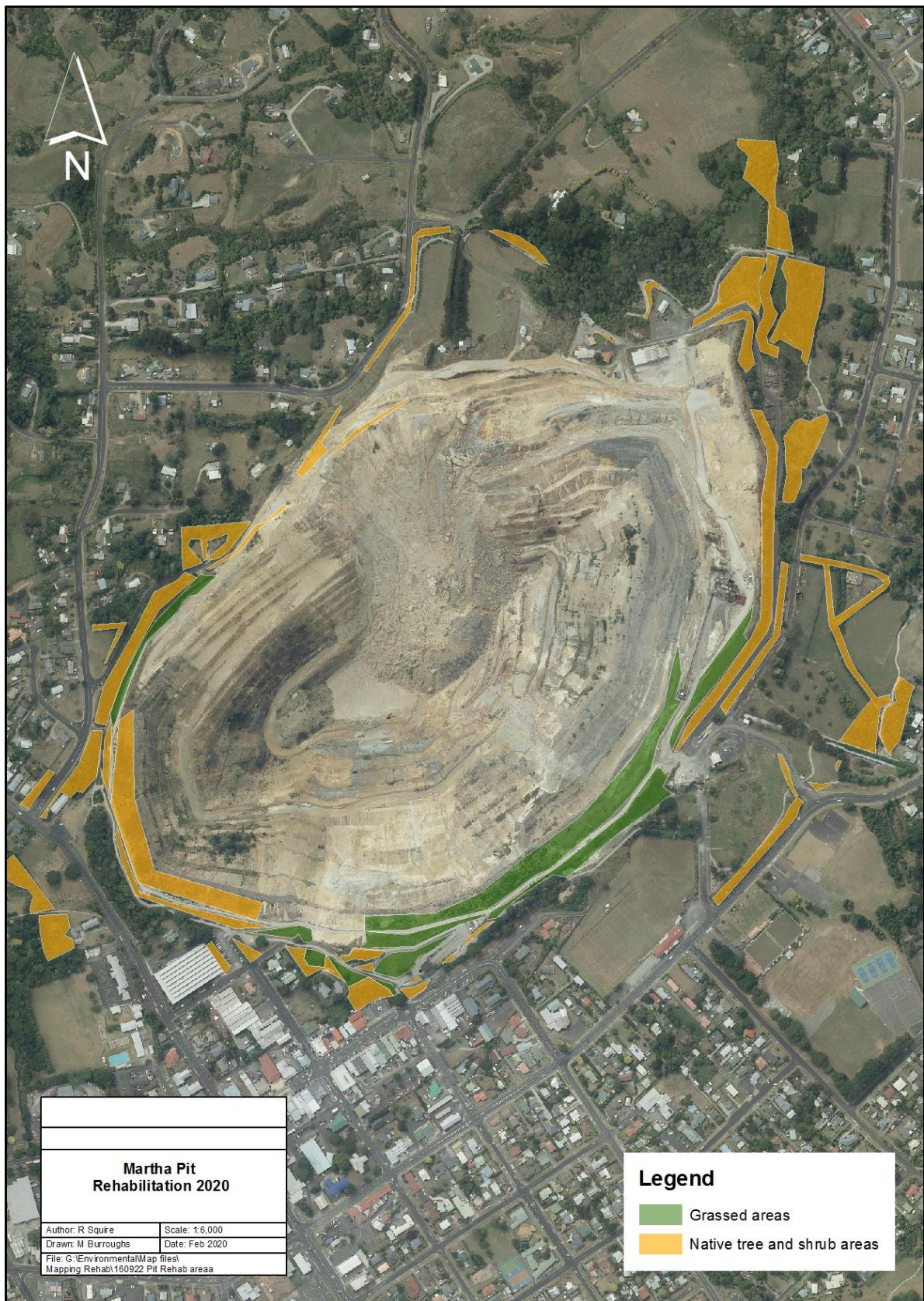
Figure 8: Rehabilitation of Open Pit and Surrounding Areas
