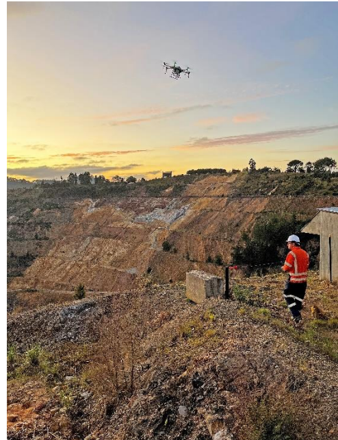
Figure 32 Dronezap are able to spray the entire Pit from above.
