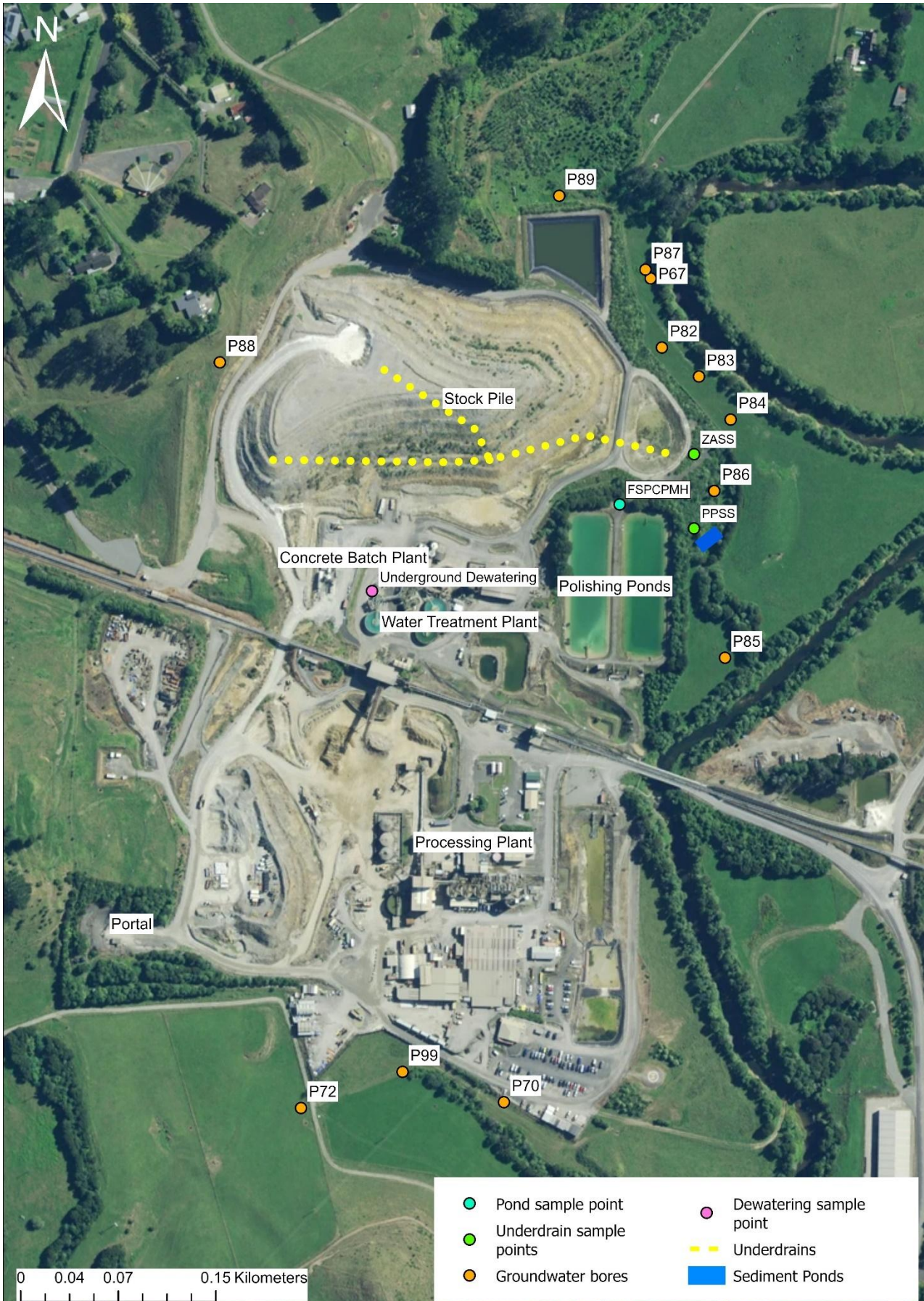
Figure 8. Mill and Favona drainage, ponds and groundwater bores.
