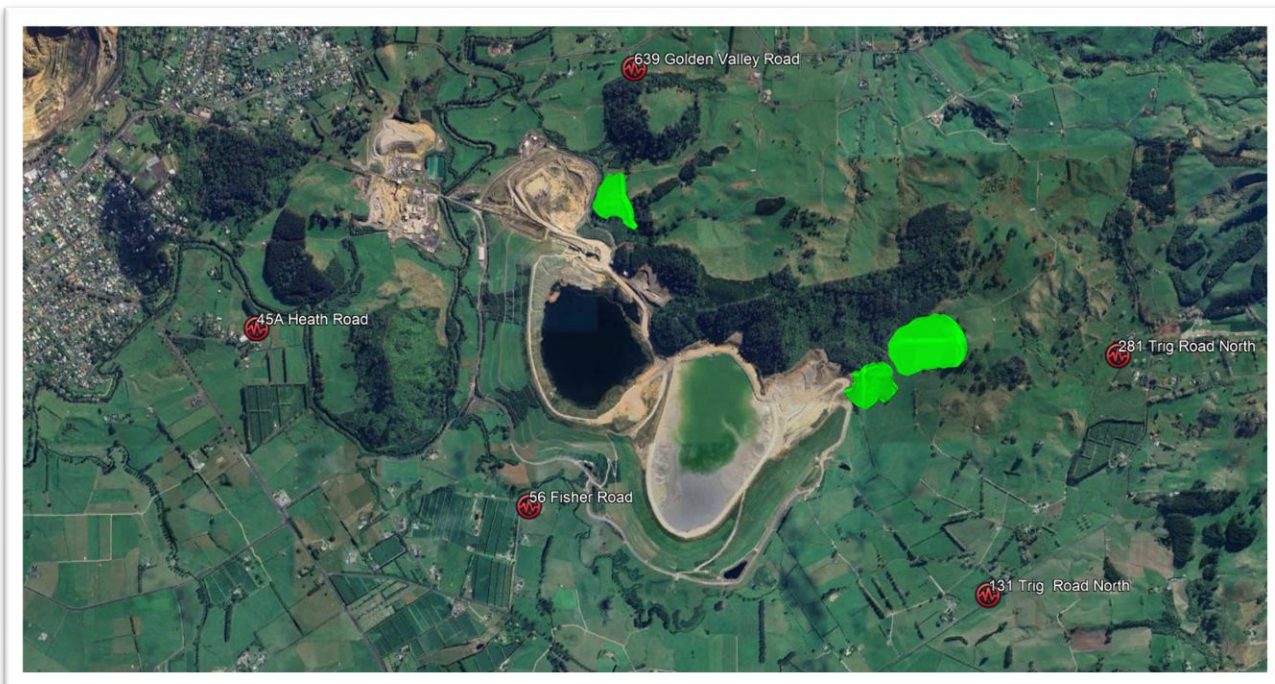
Figure 3 – Fixed Vibration Monitors for GOP and Borrow Pits
