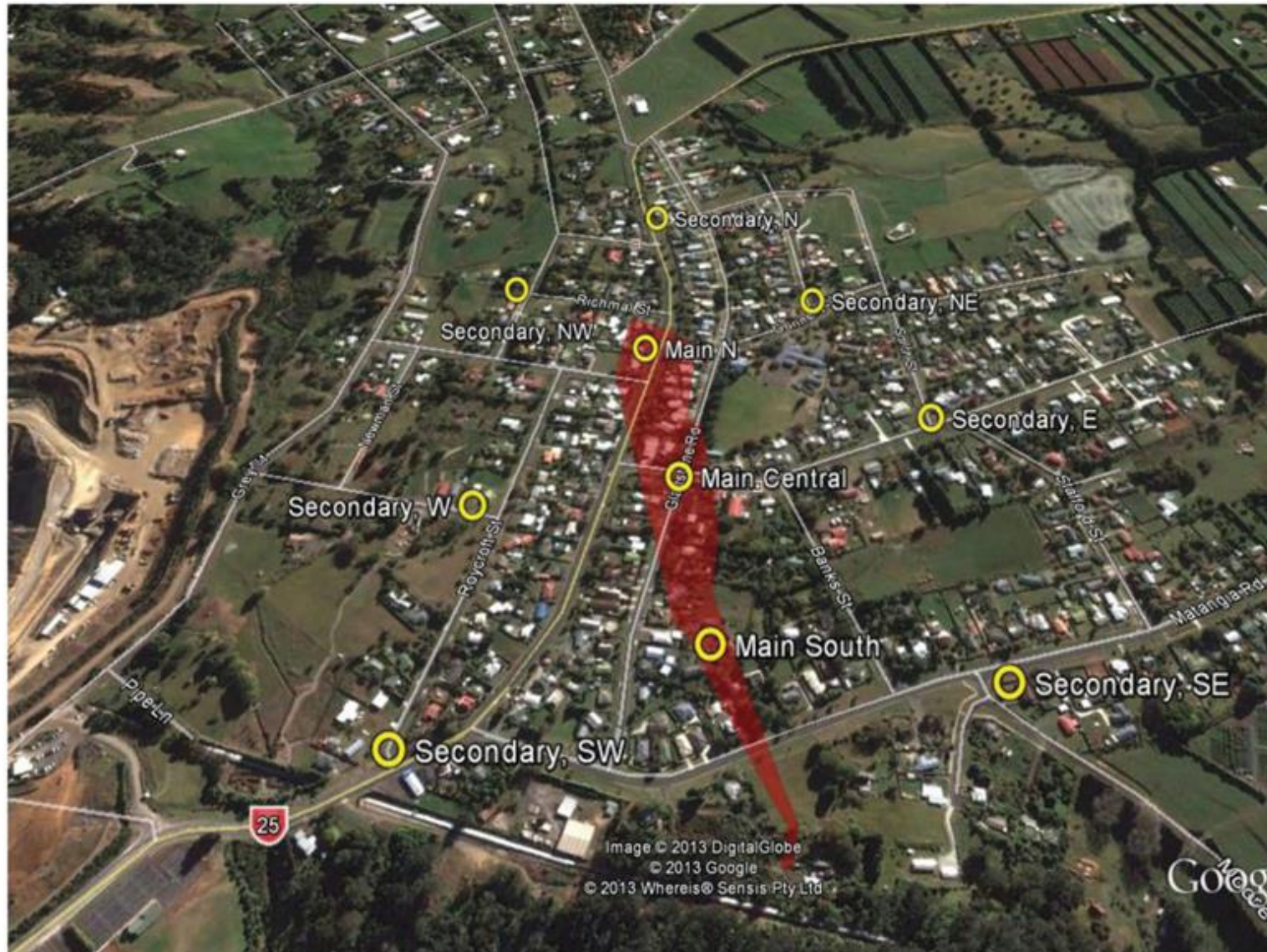
Figure 3 Position of fixed monitors
