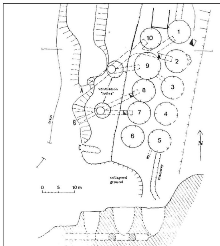
**Figure 1. Layout and Numbering of Union Hill Kilns**
