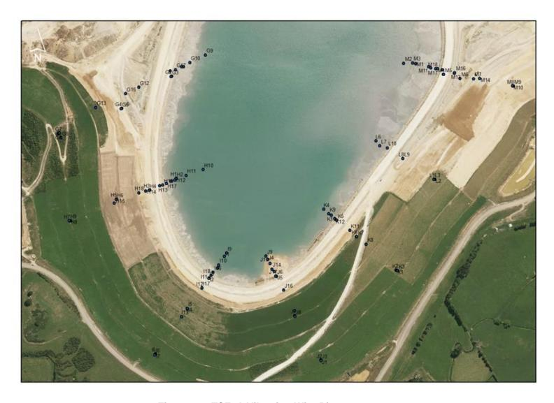
Figure 2 TSF1A Vibrating Wire Piezometers
