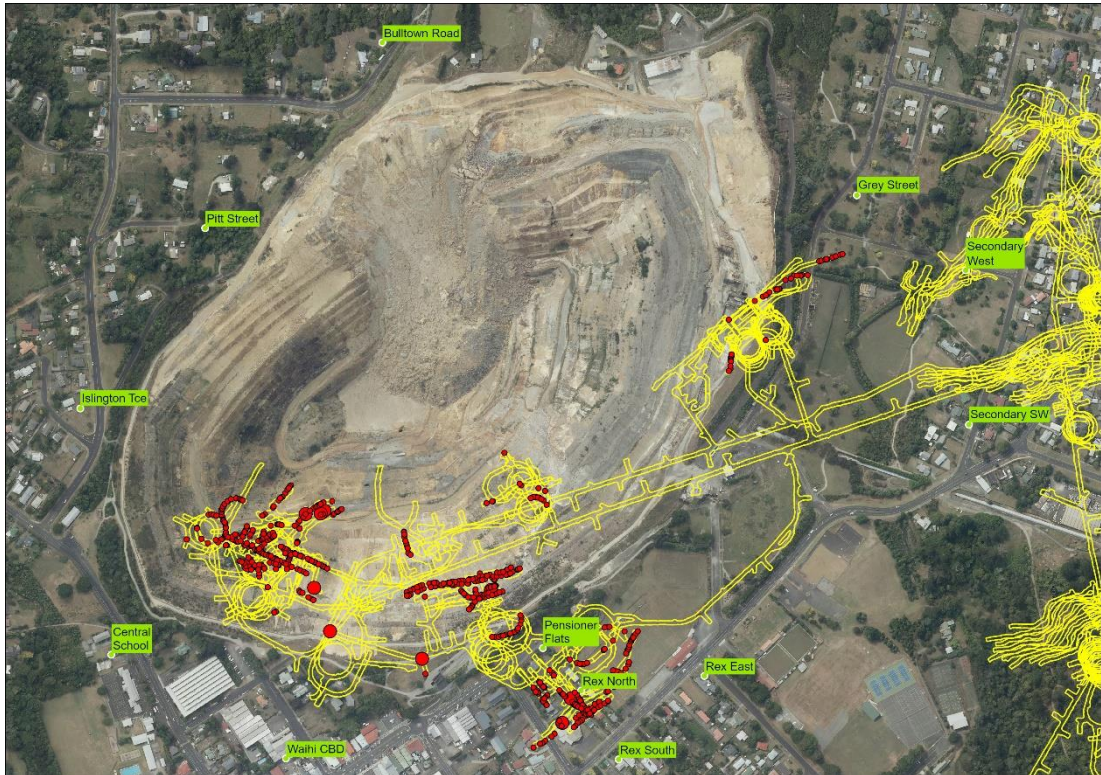
Figure 1. Vibration Monitor & Blast Locations – Project Martha
