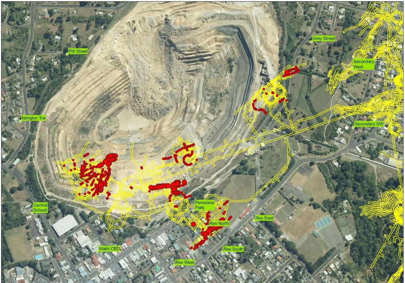
**Figure 1. Vibration Monitor & Blast Locations – Project Martha**
