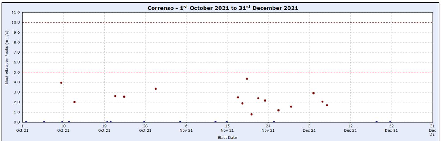
**Figure 5. Maximum Peak Vibration Levels – Correnso/SUPA Operations**
