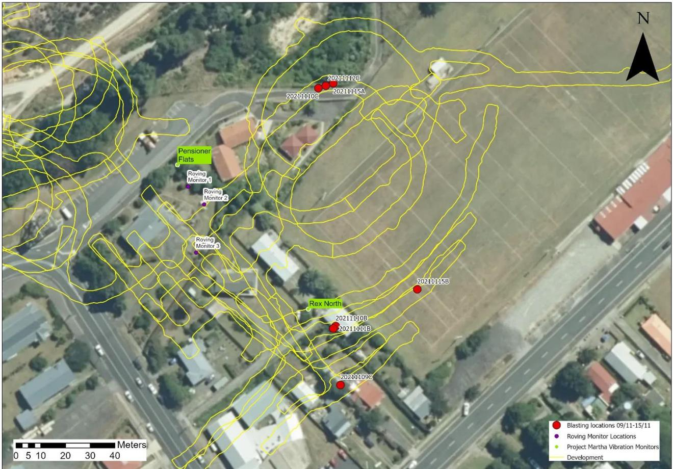
Figure 10. Pensioner Flats roving monitor locations, long-term monitoring locations and blast locations, 09-15 November 2021
