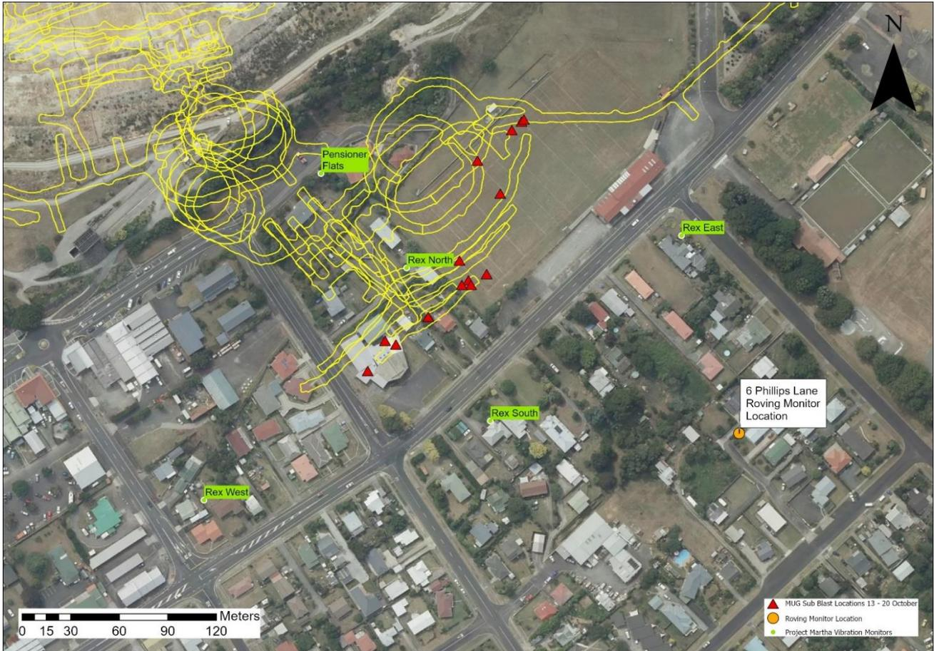
**Figure 9. Phillips Lane roving monitor location, long-term monitoring locations, and blasting locations 13-20 October**
