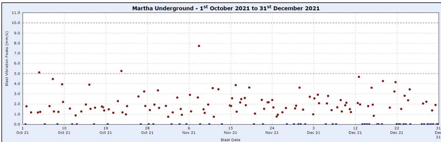
**Figure 4. Maximum Peak Vibration Levels – Martha Underground Operations**
