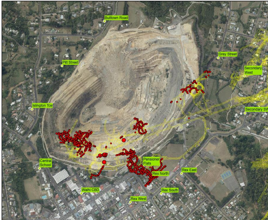
Figure 1. VMS Monitor & Blast Locations – Project Martha
