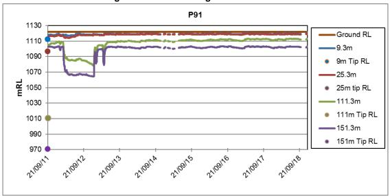
Figure 11: P91 Vibrating Wire Piezometer
