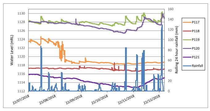
Figure 20: Water Levels in North Wall Piezometers
