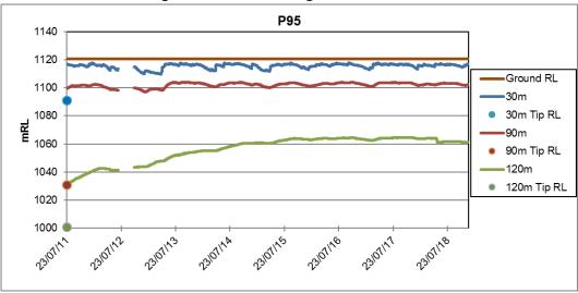
Figure 15: P95 Vibrating Wire Piezometer
