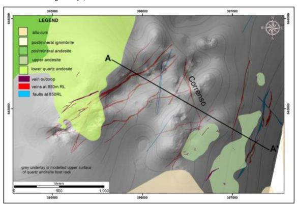
Figure 1(b) Veins and faults from around Martha & Favona mines, showing projected Correnso (J Hobbins, OGNZL Exploration Dept.).
