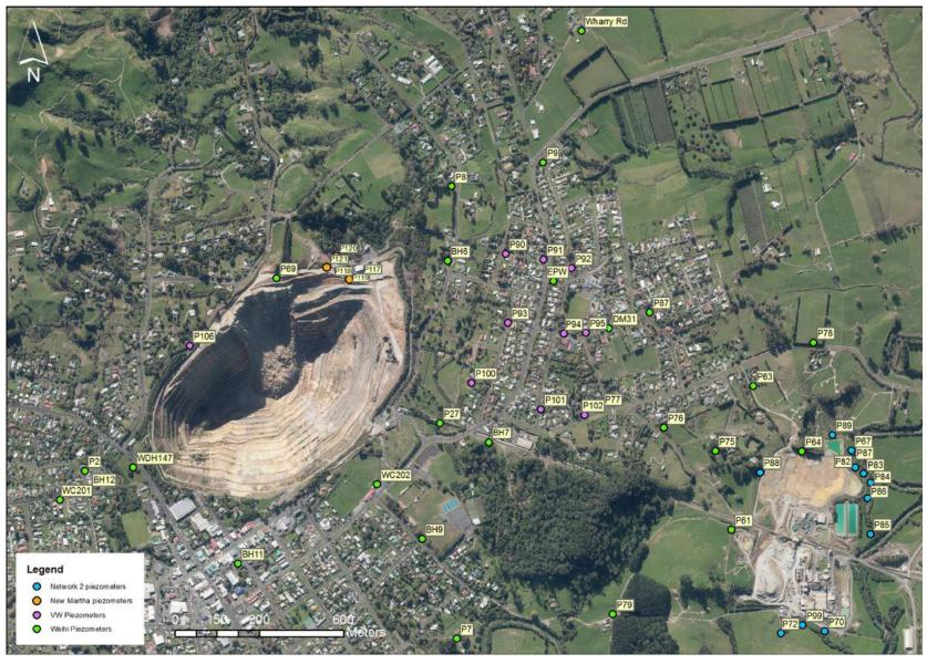
Figure 2: Piezometer Location Plan
