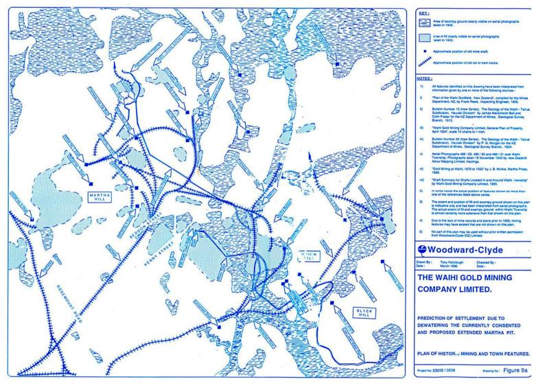
Figure 1 WWC (1996) Plan of Mining Features, Areas of Fill and Swamy Ground
