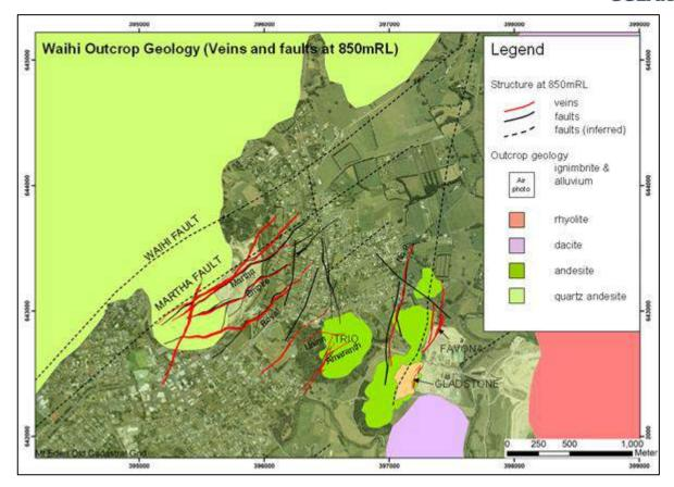
Figure 1(c) Faults and geology at 850 m RL showing main structural elements
