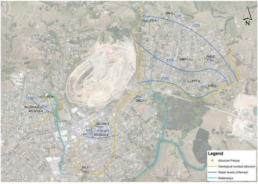
Figure 3: Alluvium Water Level Contours
