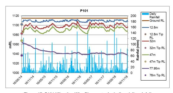
Figure 17: P101 Vibrating Wire Piezometer including daily rainfall
