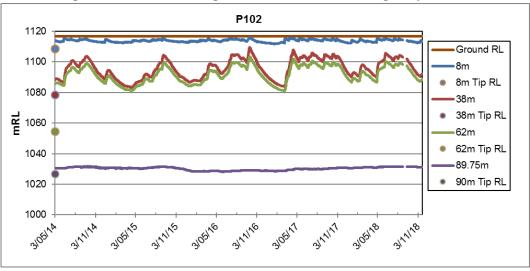
Figure 18: P102 Vibrating Wire Piezometer
