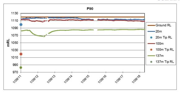
Figure 10: P90 Vibrating Wire Piezometer
