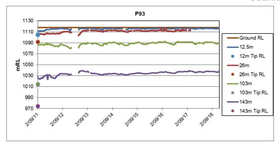
Figure 13: P93 Vibrating Wire Piezometer
