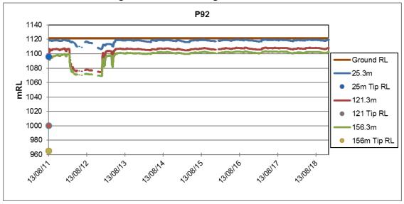
Figure 12: P92 Vibrating Wire Piezometer
