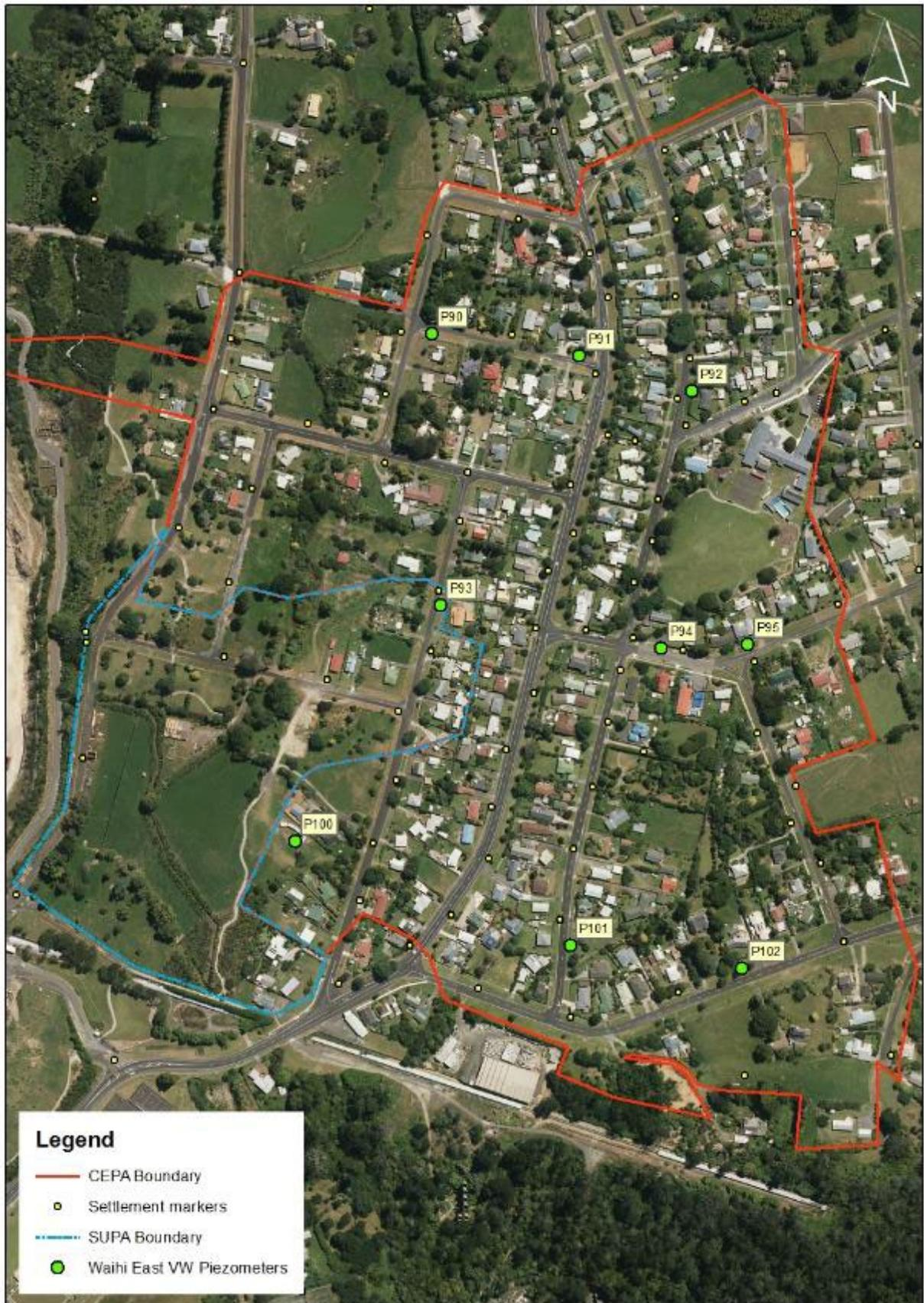
Figure 10: Waihi East Vibrating Wire Piezometers and Settlement Markers
