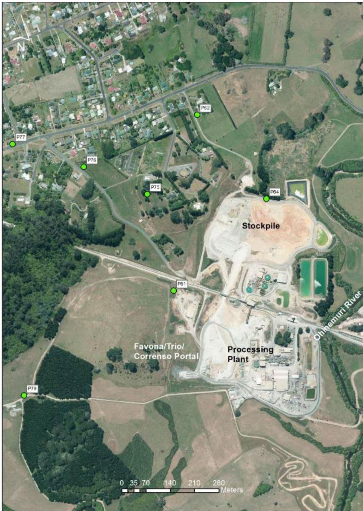
Figure 9: Location of post closure monitoring piezometers (Network 3)
