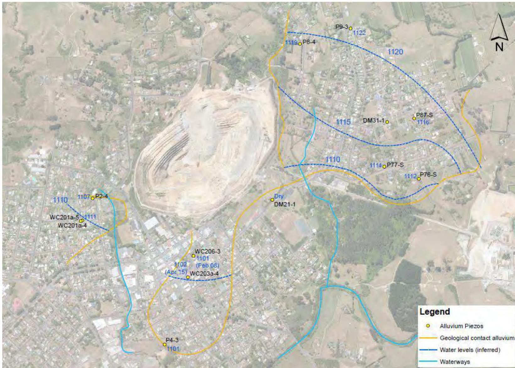
Figure 3: Alluvium Water Level Contours
