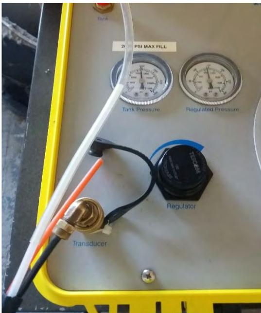
1. The twin-tubing from the transducer contains a black tube, nitrogen fill, and a clear (whitish) tube for the return flow. Both Ends have quick-connect plugs (female) to connect to the piezometer male ends. Connect black to black and white to white.
