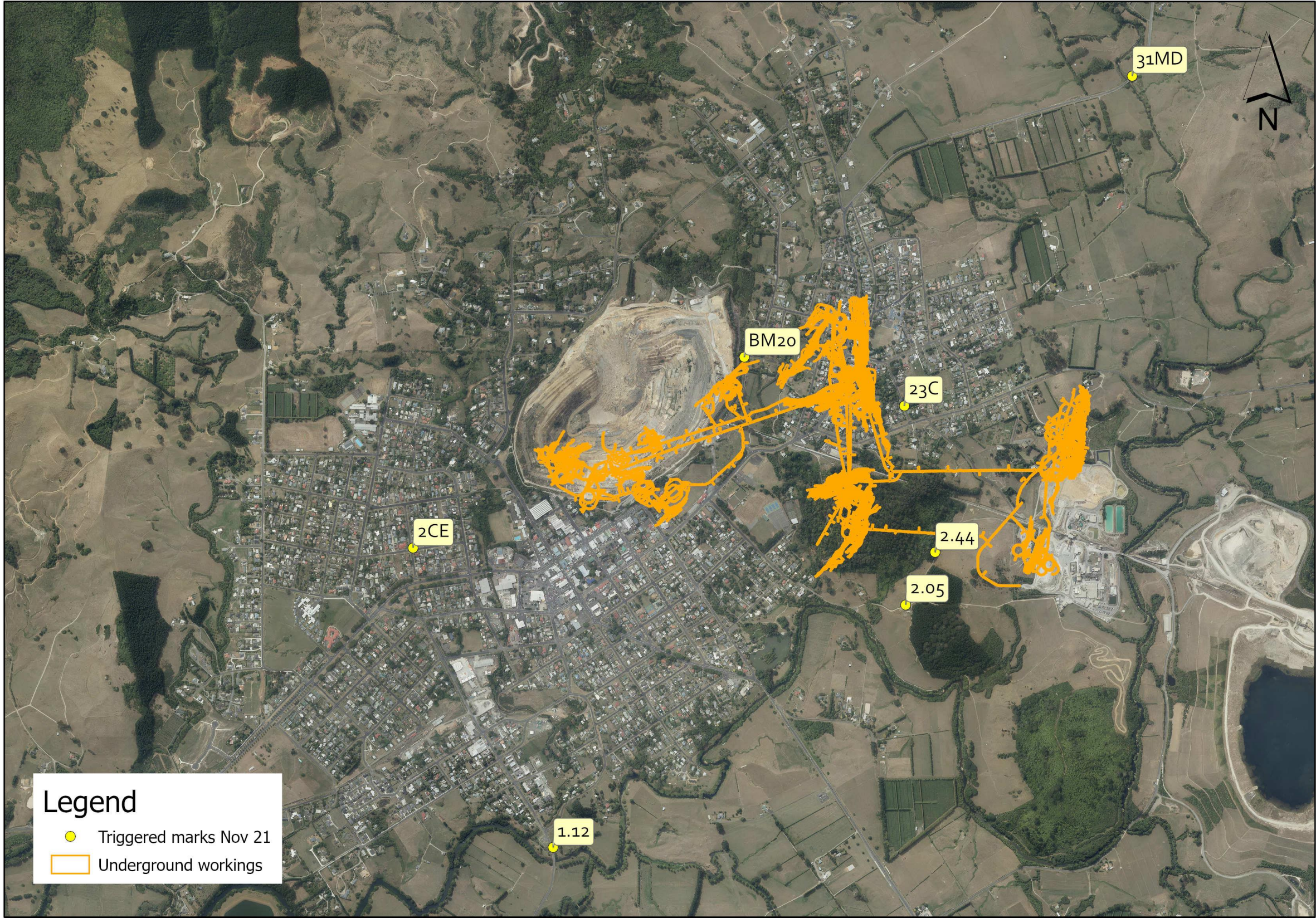
Figure 33: Triggered settlement marks Nov 2021
