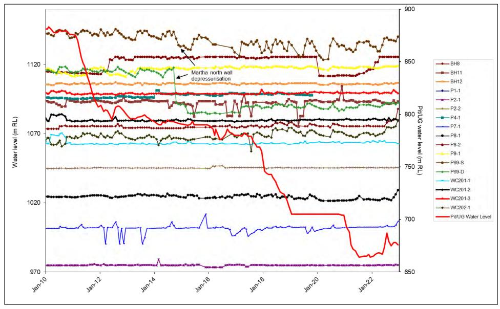
Figure 17. Andesite water level trends (excl. VW piezometers).
