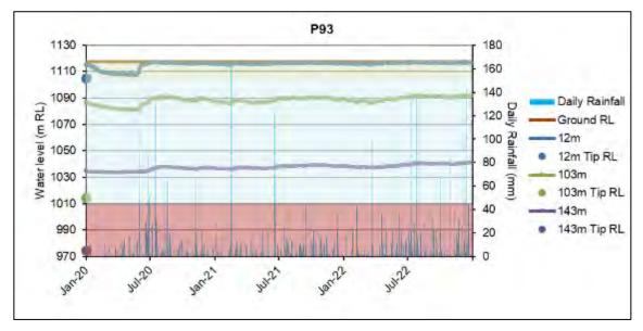
Figure 29. P93 vibrating wire piezometer.
