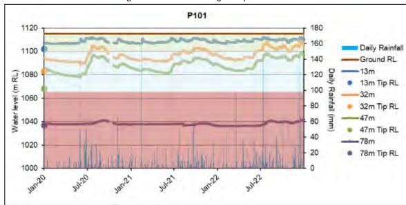
Figure 33. P101 vibrating wire piezometer.
