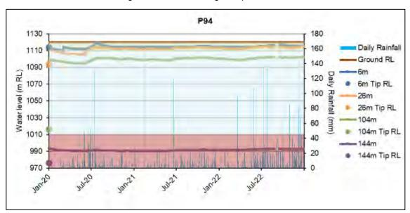
Figure 30. P94 vibrating wire piezometer.
