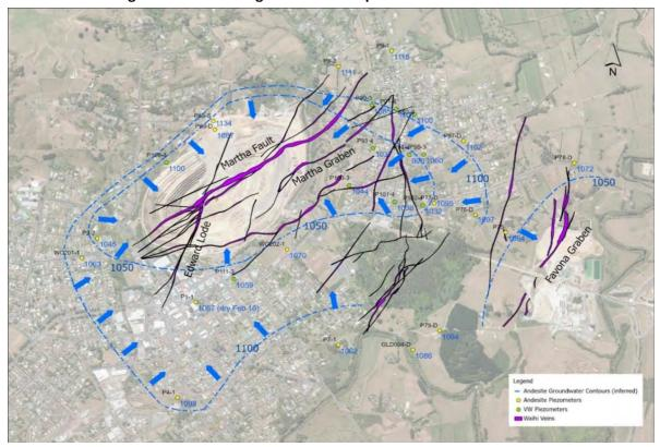
Figure 5 Andesite Piezometric Surface
