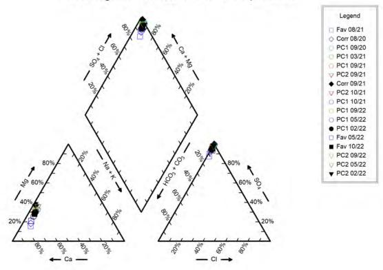
Figure 52: Underground Comparison Water Piper Trilinear Diagram
