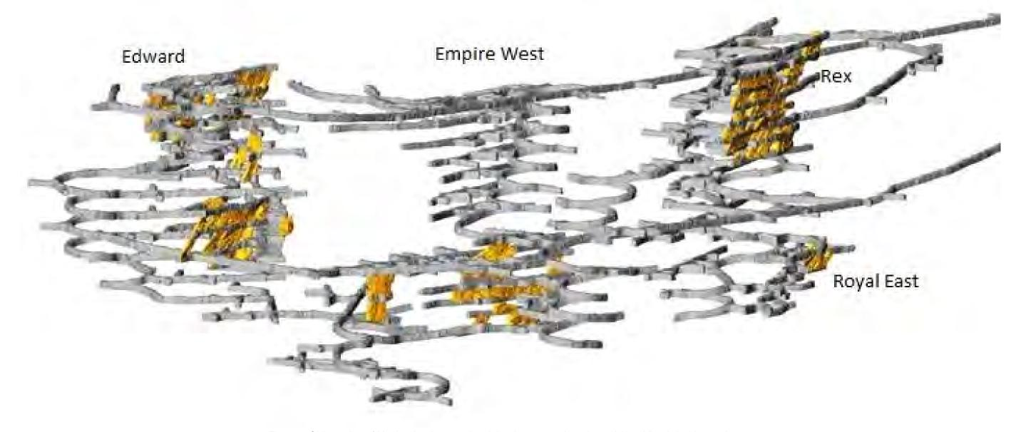
Figure 5. Oblique view of Martha showing completed development and stoping activities. View is looking northeast.
