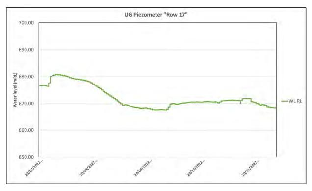
Figure 23: Underground piezometer water level
