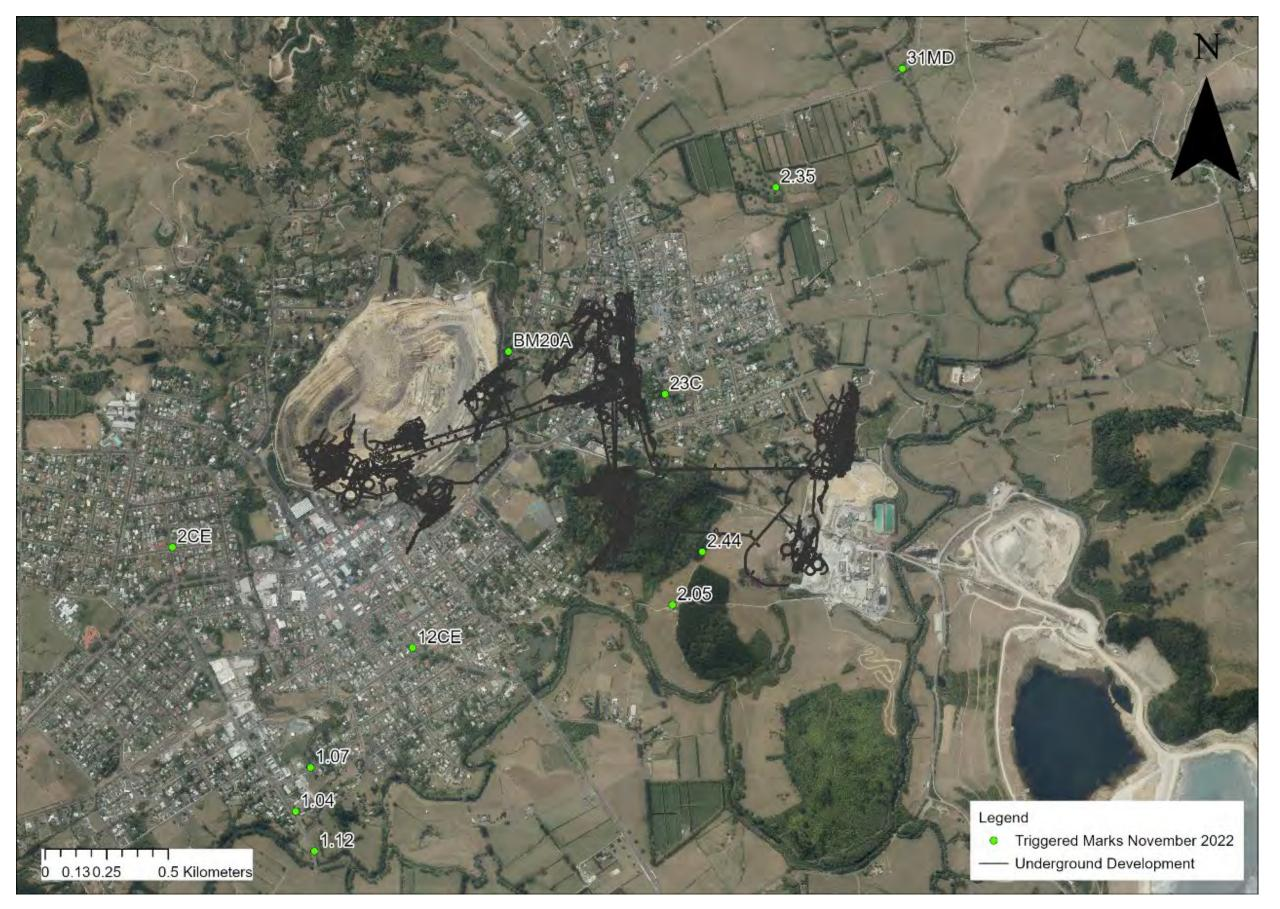
Figure 40: Triggered settlement marks Nov 2022
