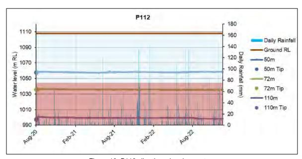
Figure 19. P112 vibrating wire piezometer.
