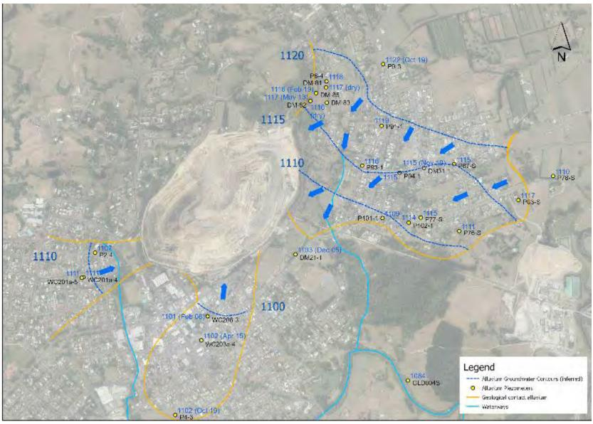
Figure 11. Alluvium water level contours.
