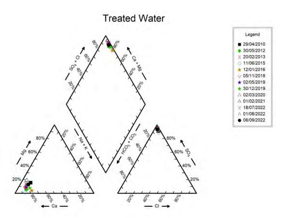
Figure 53: Treated Water Piper Trilinear Diagram
