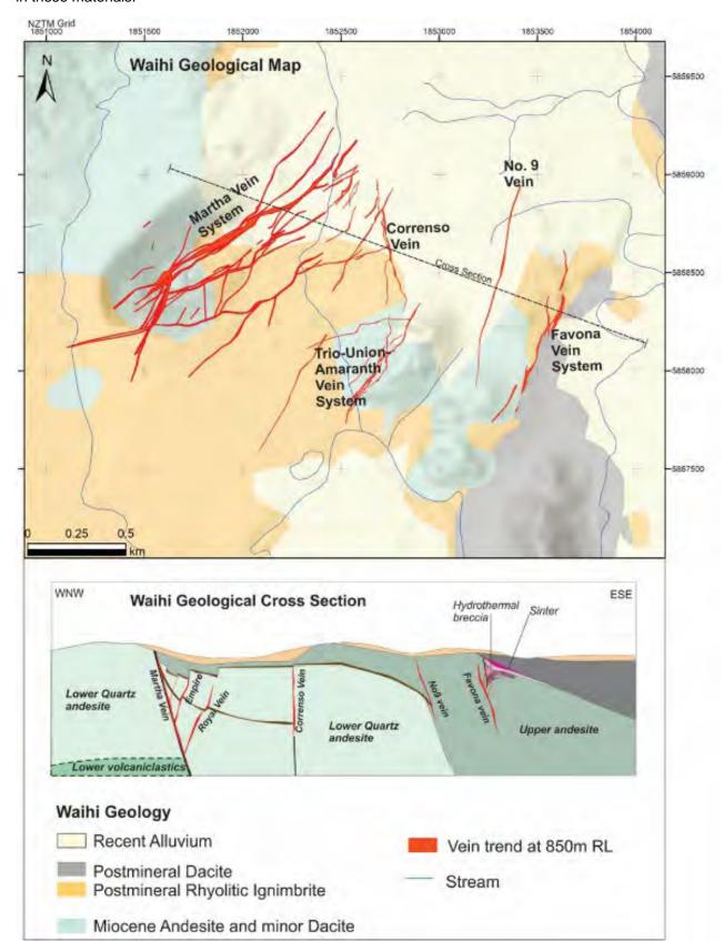
Figure 2. Geological map and cross section of the Waihi area showing the distribution of quartz veining and dominant geological rock units.
