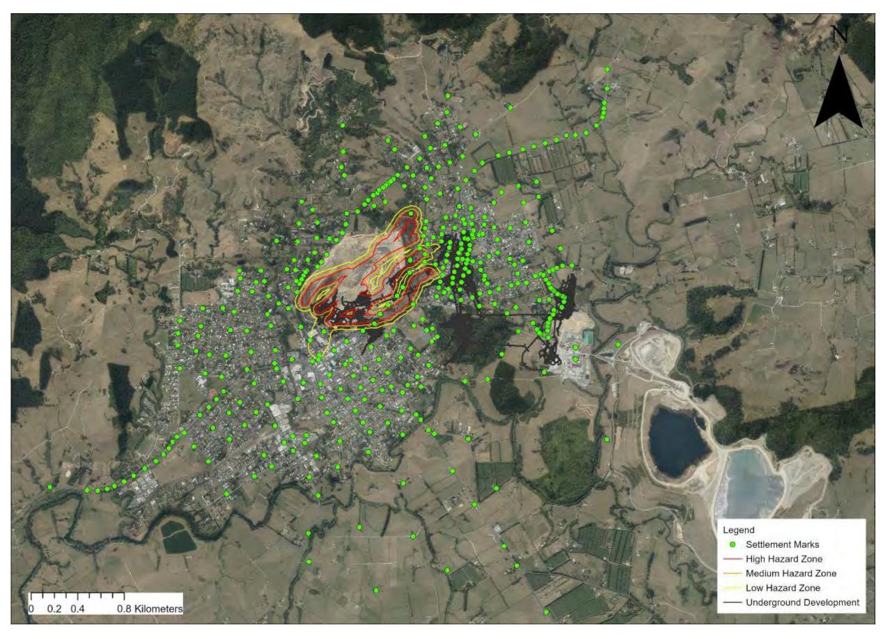
Figure 38: Settlement Marker Location Plan & Hazard Zones
