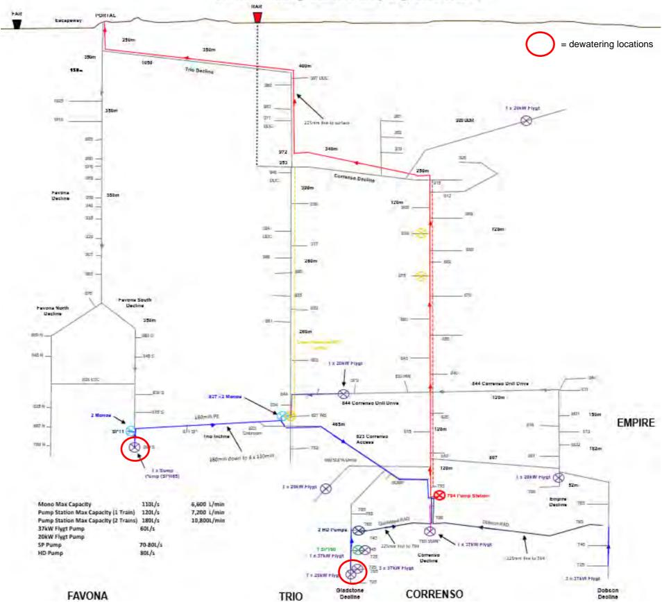
Figure 8. Correnso, Trio and Favona pumping schematic - December 2022.
