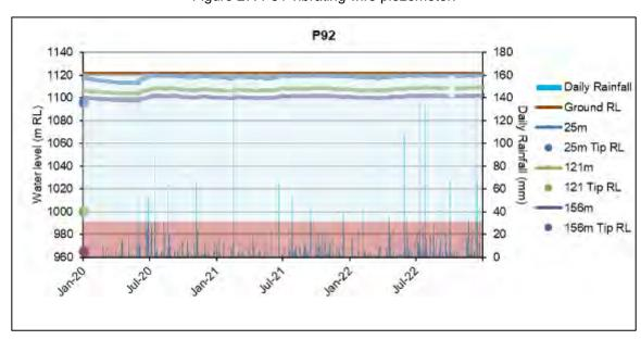
Figure 28. P92 vibrating wire piezometer.
