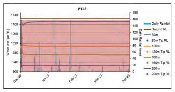
Figure 21. P123 vibrating wire piezometer.
