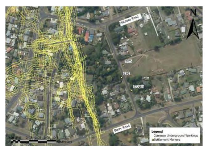
Figure 47: Correnso Tilts and Underground Workings
