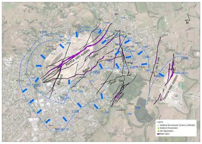
Figure 16. Upper andesite water level contours.
