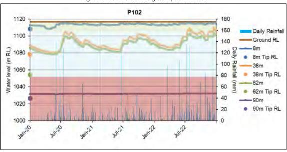
Figure 34. P102 vibrating wire piezometer.
