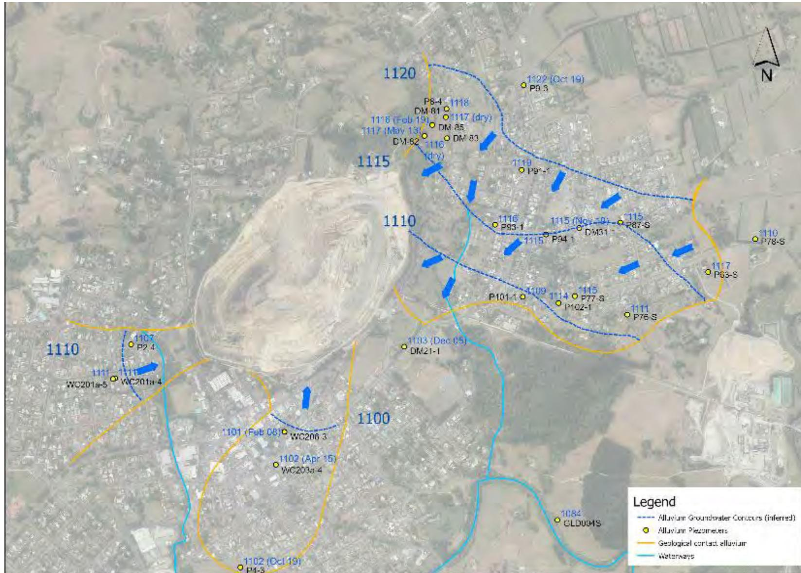
Figure 11. Alluvium water level contours.
