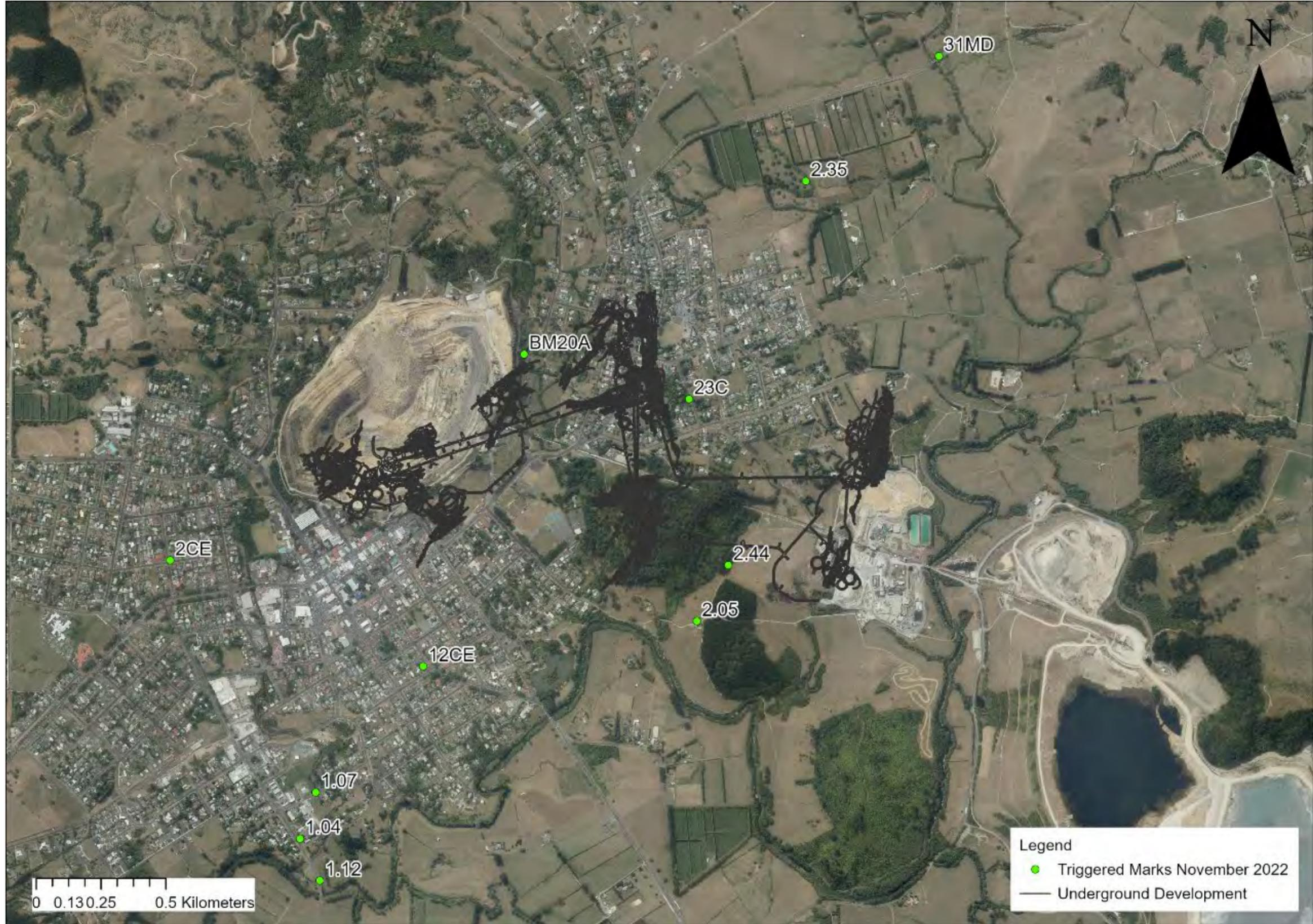
Figure 40: Triggered settlement marks Nov 2022
