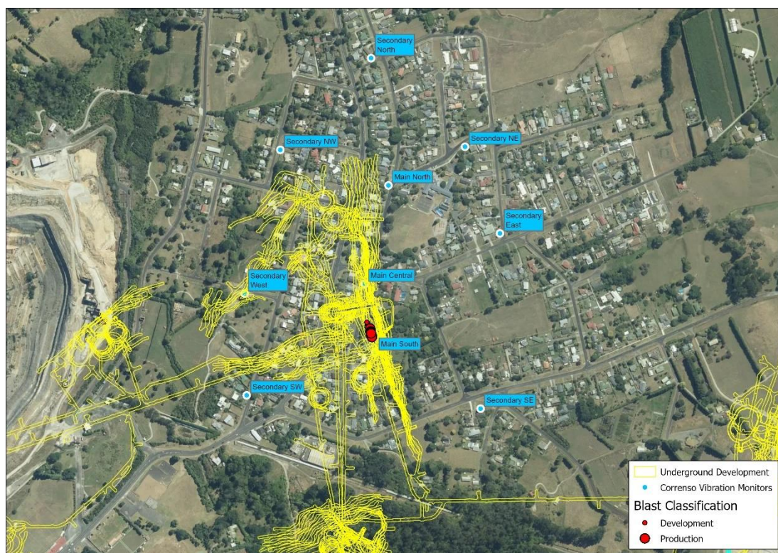
Figure 3. Vibration Monitor & Blast Locations – Correnso
