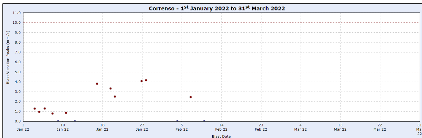
Figure 5. Maximum Peak Vibration Levels (Production and Development) – Correnso
