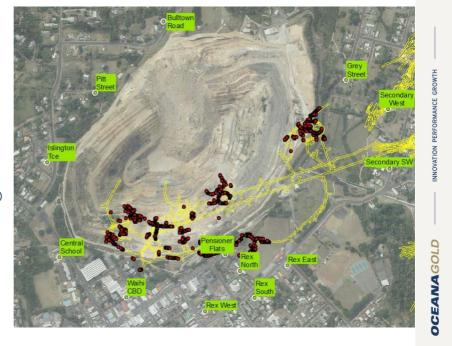
Russell said: On this picture we are overlaying the development blasting. You can see how the drives that have gone into the pit are completed now and we're back into these areas. As Jol said we're working up and down through the areas to join up the different workings and working towards the development headings. The dots are all the vibration monitors. In the last 6 months we've had 330 blast events. We try and get every
