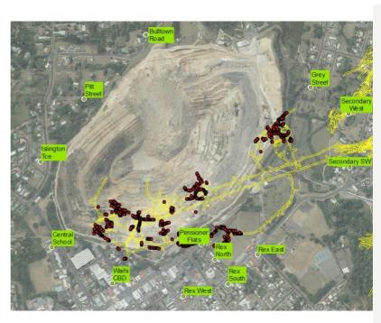
Russell said: On this picture we are overlaying the development blasting. You can see how the drives that have gone into the pit are completed now and we're back into these areas. As Jol said we're working up and down through the areas to join up the different workings and working towards the development headings. The dots are all the vibration monitors. In the last 6 months we've had 330 blast events. We try and get every
