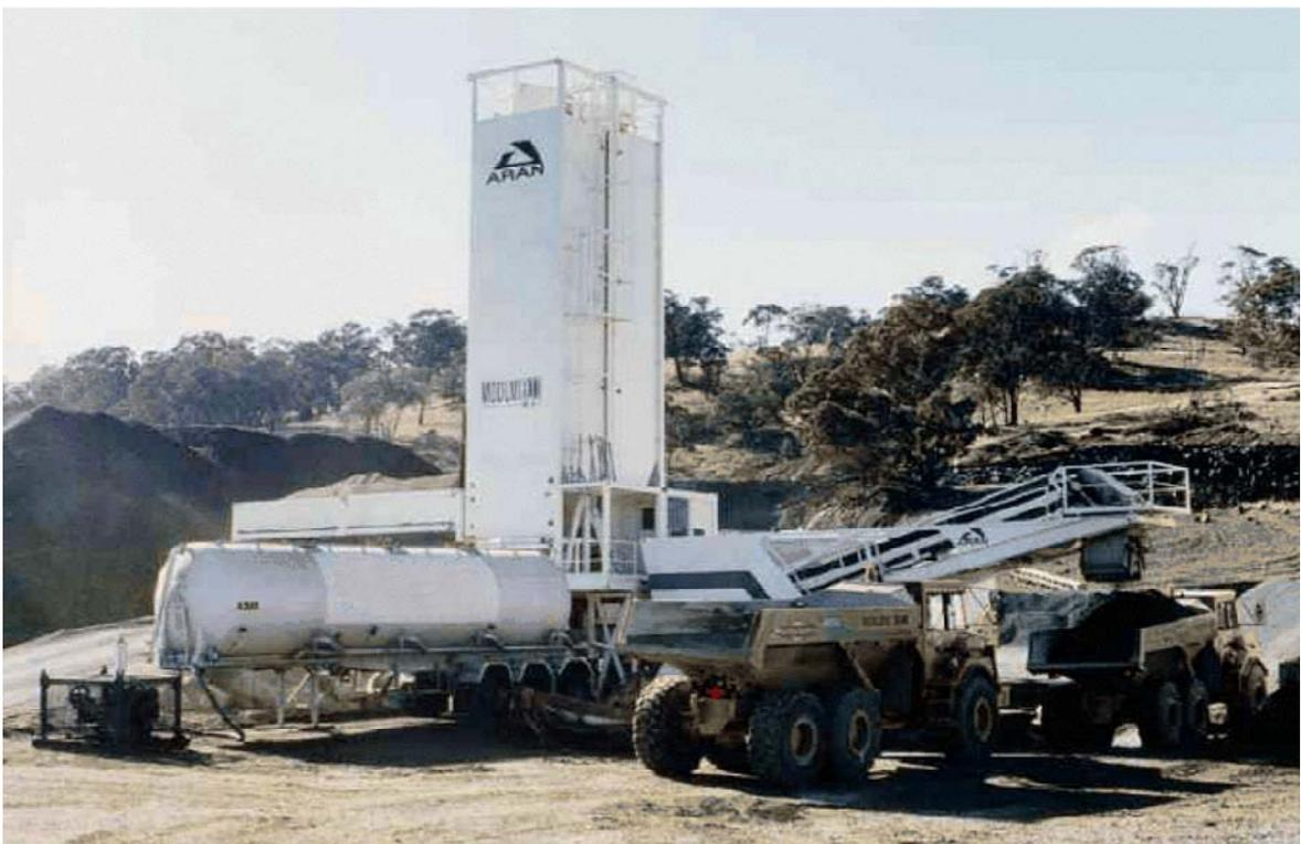
Figure 6: Photograph of a Typical Batching Plant<sup>10</sup>
