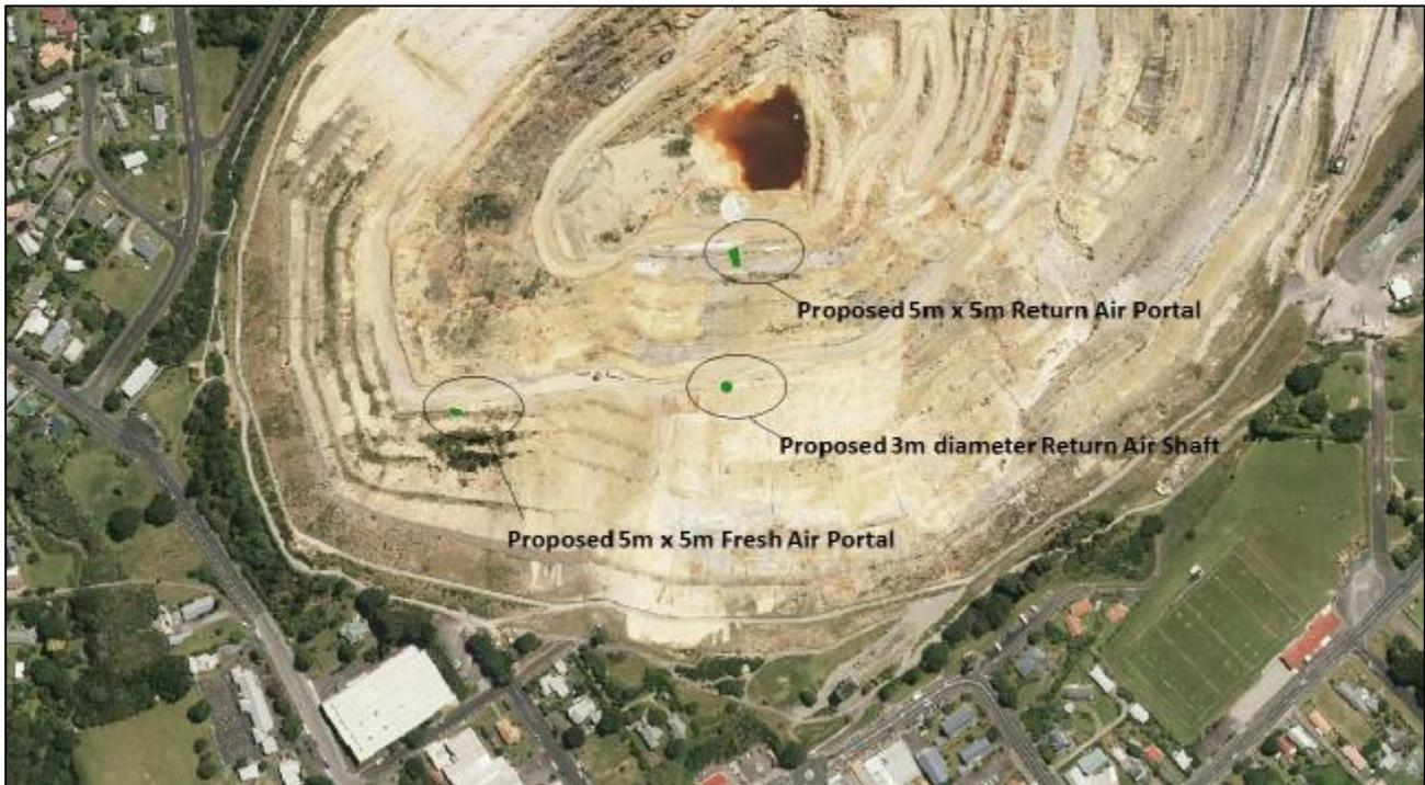
Figure 2-3 Proposed surface ventilation structures associated with MUG in Martha Pit (Source OGNZL)
