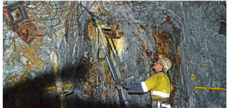
Using an 'airleg' as part of narrow vein mining.
