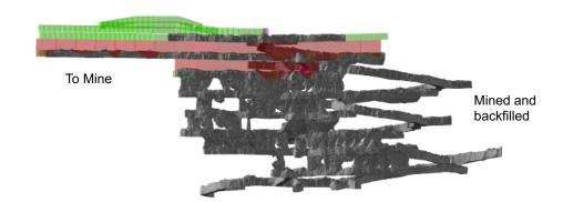
Dave T said: Last month that level hadn't been mined. We've stoped that now. All these areas are stoped up to level 4. This is level 3. We're developing level 2 so we're pretty much developing the last level in Rex which is level 2. We're about here at the moment so we'll just finish this off and we'll start stoping towards the end of the year. There's not much left to go in Rex. We'll finish that one more level of stoping and then just put some cut and fill over the top.
